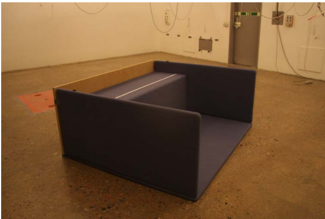
Picture 8 – Sofa Sound Booth was also tested placed with the back against the floor and a board covering the bottom. The measurement corresponds to a placement of the Sofa Sound Boot at a wall or similar.
