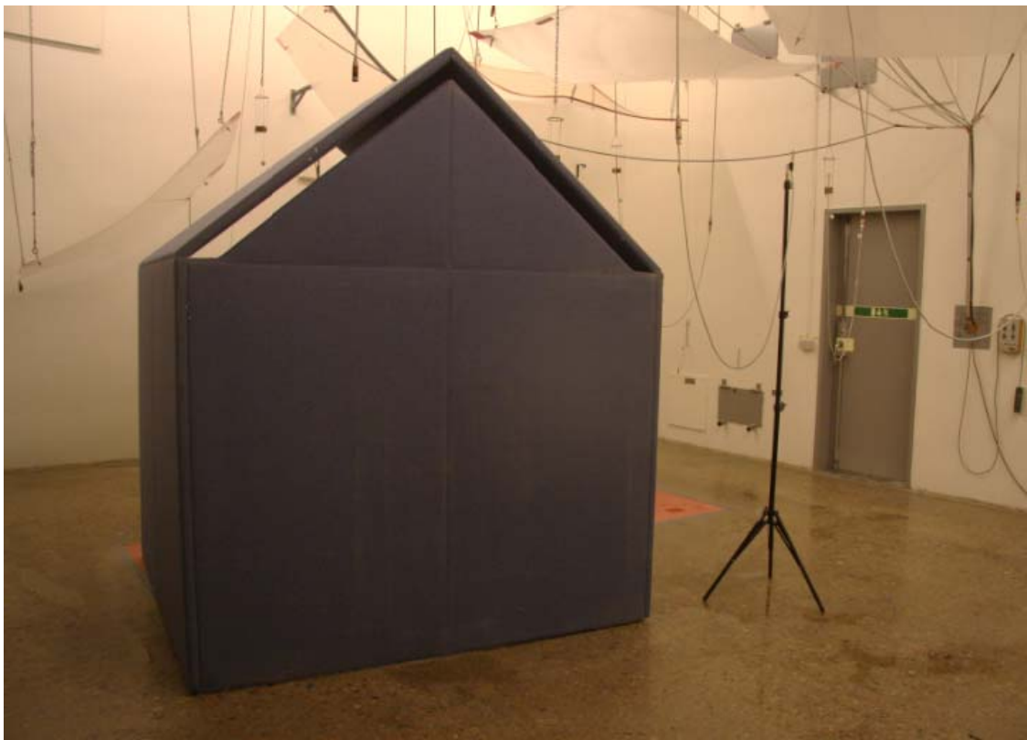
Picture 4 – One test object type The Hut was tested in three different positions. The Hut is seen from the back.
