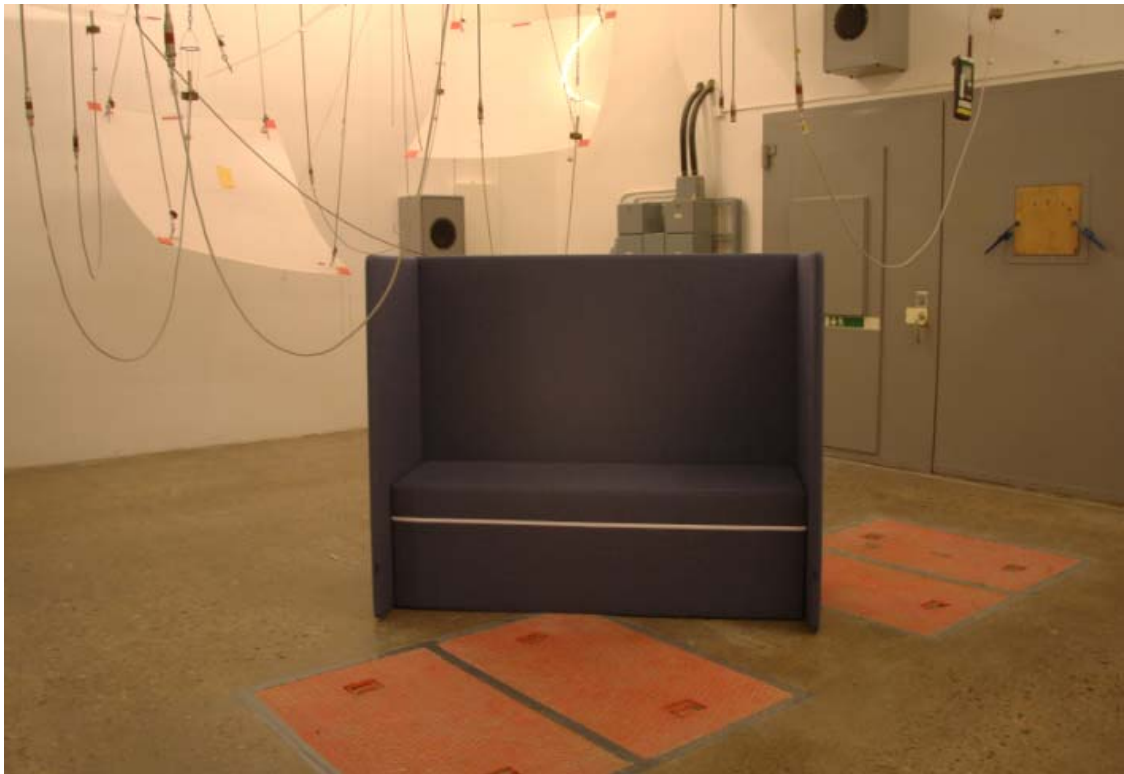
Picture 7 – One test object type Sofa Sound Booth was tested in three different positions. The Hut is seen from the back.
